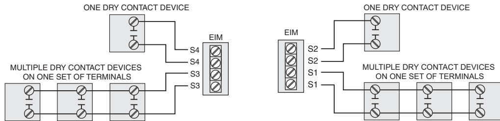
Fig. 157. Wiring dry contact devices.
