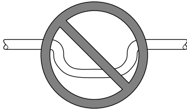
Fig. 19 – Insufficient Condensate Trap
