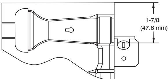
**Fig. 50 – Igniter Position - Top View**
