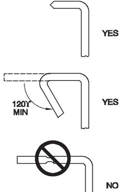
**Fig. 18 – Duct Flanges**
