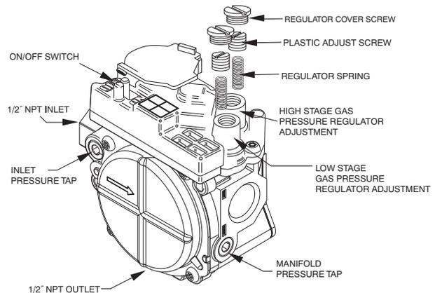
**Fig. 22 – Redundant Automatic Gas Control Valve**
