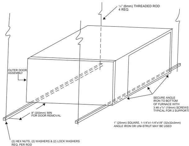
**Fig. 15 – Horizontal Unit Suspension**
