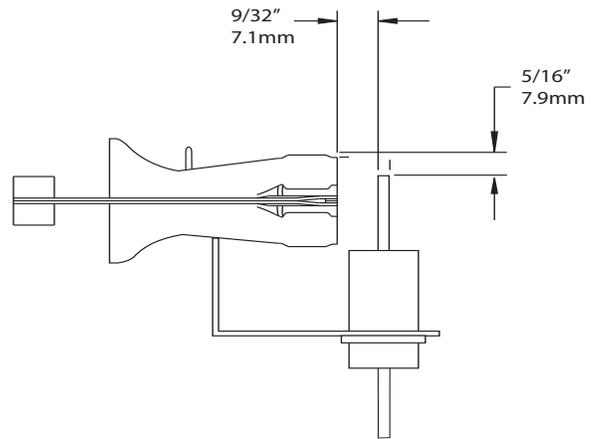
**Fig. 51 – Igniter Position - Side View**
