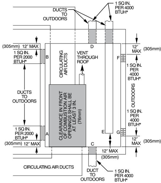
\* Minimum dimensions of 3 in. (76 mm).
