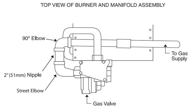
**Fig. 23 – Burner and Manifold**
