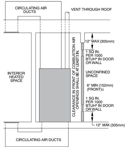
\* Minimum opening size is 100 in.2 with minimum dimensions of 3 in. (76 mm).
