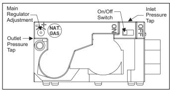
FIGURE 11: Modulating Gas Valve
