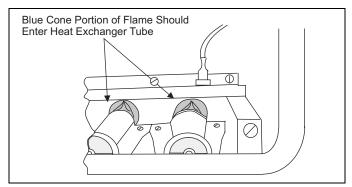
FIGURE 7: Burner Flame Drawing (Upflow Configuration Shown)
