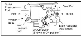
FIGURE 9: Single Stage Gas Valve
