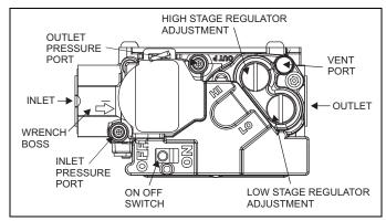
FIGURE 10: Two-Stage Gas Valve
