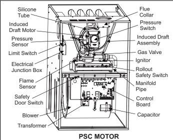
FIGURE 3: Component Location - 80% Modulating PSC Models
