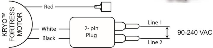
CW Rotation - Connect 2-pin (White and Black wires) plug only CCW Rotation - Add Red wire to L1 or L2
