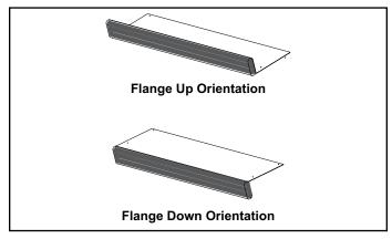
Figure 4. Positioning Divider Panel
