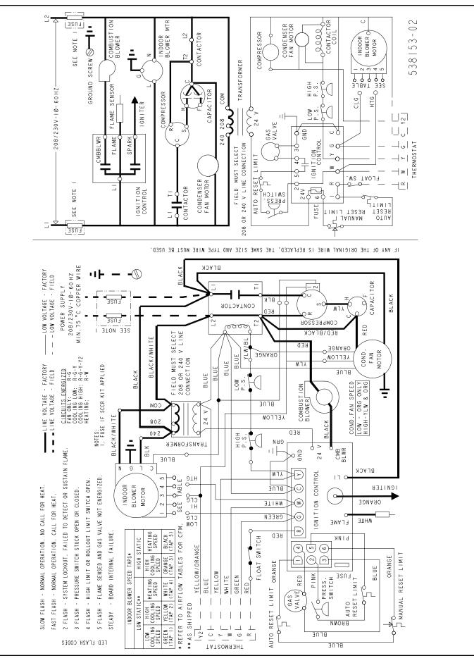
Figure 14. Wiring Diagram - MGE 3 Ton
