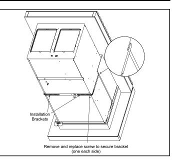
Figure 7. Securing Unit
