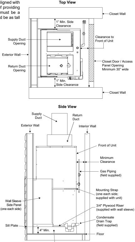
Platform (field supplied) - Unit must be supported by platform, which must be
