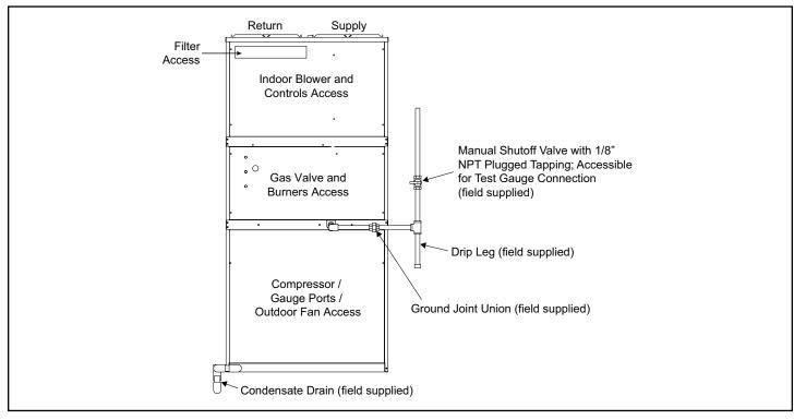
Figure 9. Gas Supply Piping
