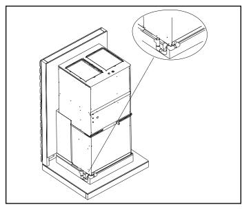
Figure 8. Condensate Drain Installation
