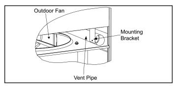
Figure 5. Locating Vent Pipe and Extension
