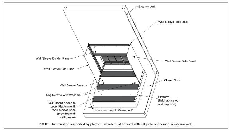
Figure 3. Wall Sleeve and Louver Kit Installation
