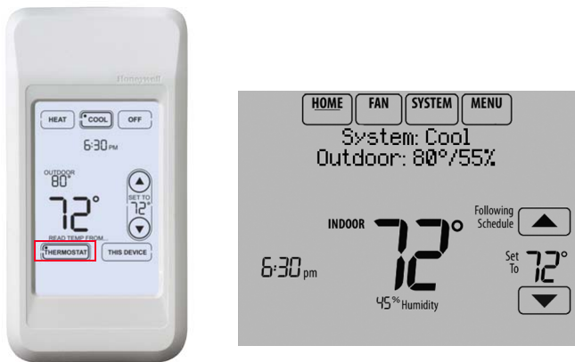
Fig. 302. Reading temperature at the thermostat.
