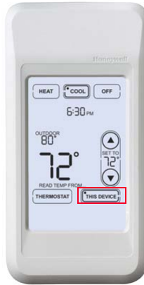
Fig. 303. Reading temperature at the Portable Comfort Control.
