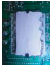
OK : Evenly applied silicon grease.
