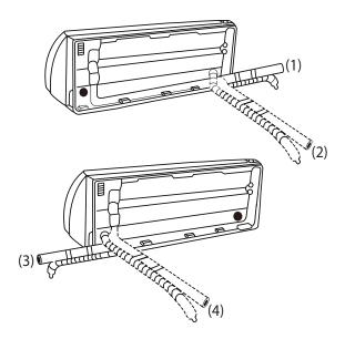
Fig. 11 —Piping Angle
