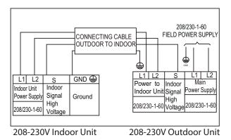
Fig. 15 —Connection Diagram Sizes 9K - 12K
