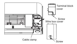
Fig. 17 —Terminal Block Location
