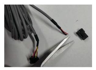
Fig. 29 —Cut the female plug and strip the wires
