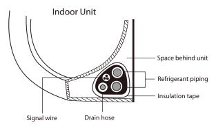
Fig. 25 —Bundle drain hose, refrigerant pipes, & signal cable
