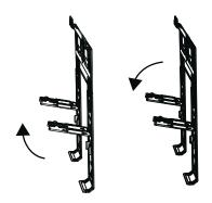
Fig. 13 —Use Holder to Prop up the Unit
