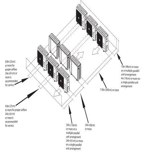
Fig. 6 – Clearances for multiple units
