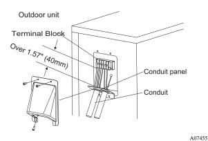
Fig. 12 - Field Wiring
