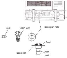
Fig. 13 - Drain Joint
