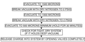
Fig. 18 – Triple Evacuation Method
