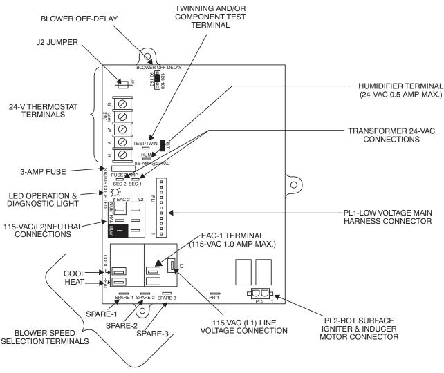
Fig. 39 - Example of Single Stage Furnace Control
