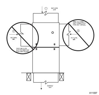
Fig. 28 - Downflow Return Air Configurations and Restrictions
