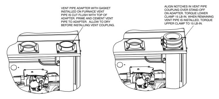
VENT PIPE FLUSH WITH ADAPTER
