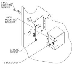
Fig. 35 – Installing J-Box (When Used)
