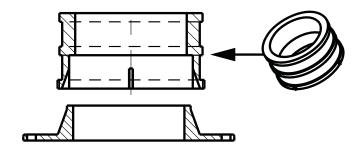
Attach gaskets to vent pipe and combustion air adapters.
