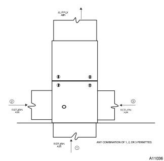
Fig. 27 - Upflow Return Air Configurations and Restrictions
