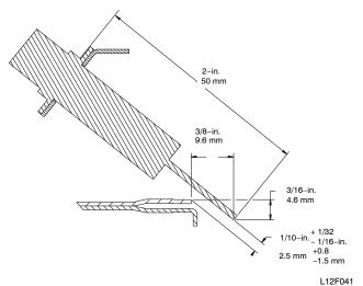
Fig. 64 - Igniter Position - Side View
