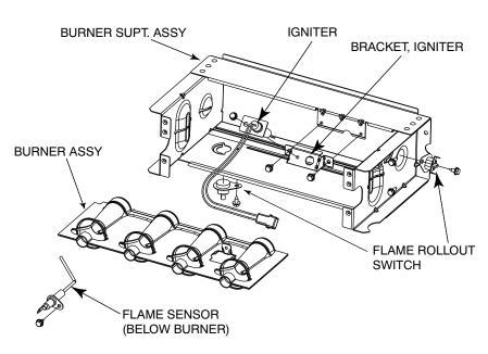
Fig. 69 - Burner Assembly
