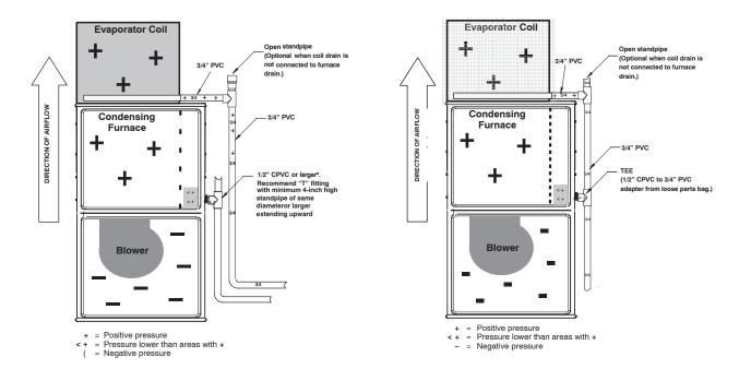
Fig. 14 - Example of Field Drain Attachment
