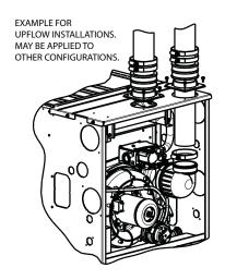
Fig. 57 - Sample Inlet Air Pipe Connection for Polypropylene Venting Systems
