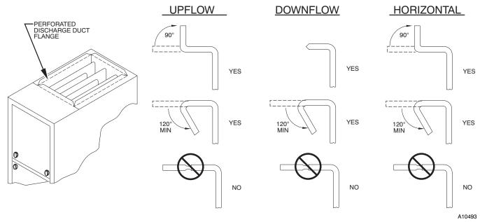
Fig. 22 - Duct Flanges
