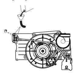
Fig. 65 - Priming Condensate Trap
