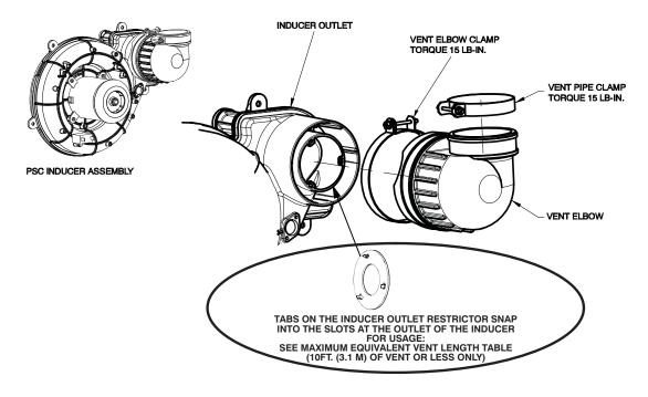
Fig. 41 – Inducer Vent Elbow
