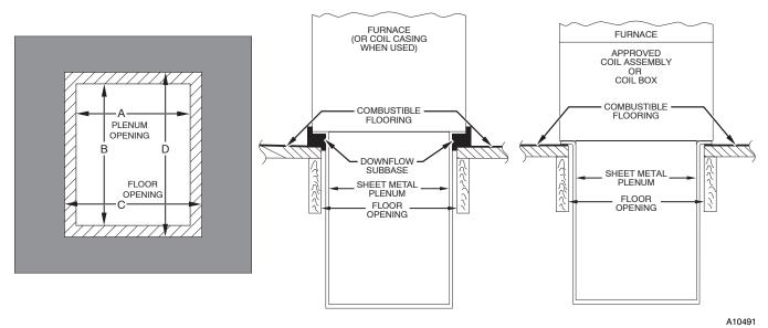
Fig. 21 - Installation on Combustible Flooring
