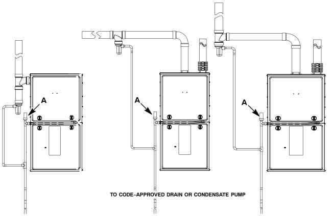
Recommend "T" fitting with 4-inch minimum height standpipe ( $\mathbf{A}$ ) of same diameter or larger extending upward.
