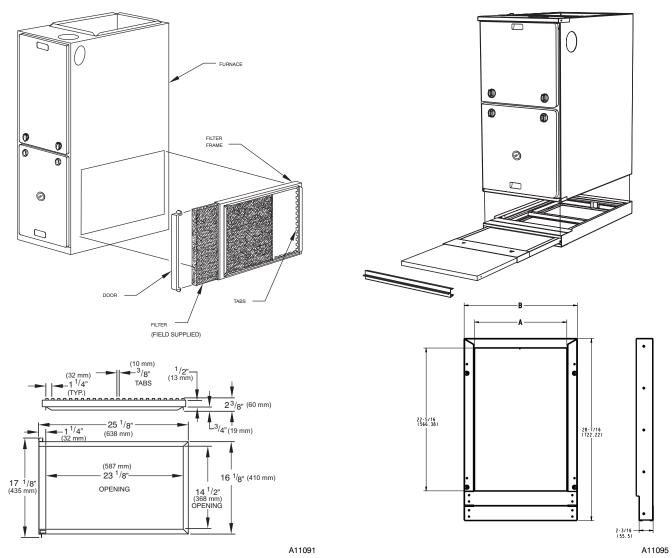
Fig. 19 - Accessory Side Filter Rack
