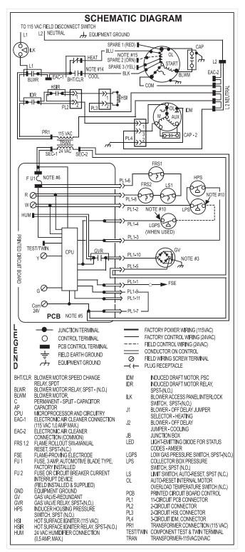
Fig. 71 - Wiring Diagram
