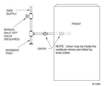
Fig. 34 - Typical Gas Pipe Arrangement
