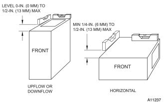
Fig. 26 - Furnace Pitch Requirements
