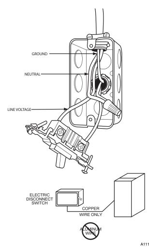
Fig. 36 – Field–Supplied External Electrical Box on Furnace Casing
