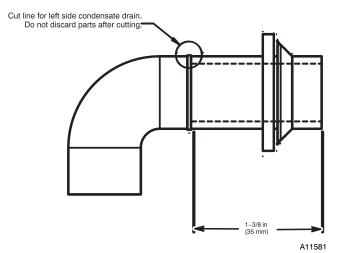
Fig. 16 - Modify Rubber Drain Elbow
