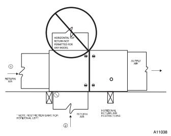
Fig. 29 – Horizontal Return Air Configurations and Restrictions
