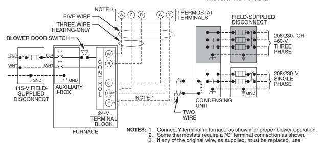
Fig. 38 - Typical Single-Stage Wiring Diagram
