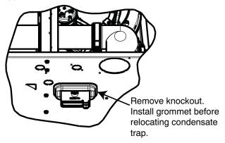
Fig. 17 - Horizontal Drain Trap Grommet
